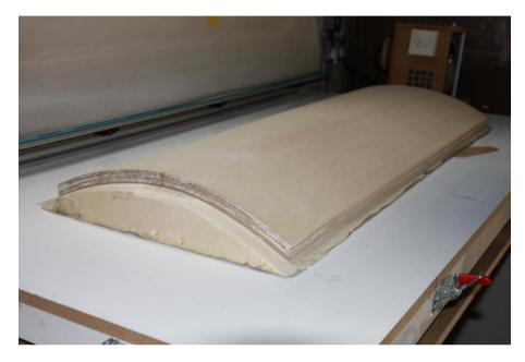
One of the side panels being laminated from multiple ply layers in a DIY vacuum former using high grade PVA glue. The glue was selected to be "lossy" so that it never sets hard but remains slightly flexible. Another way to win the battle against unwanted resonance!
