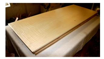
One of the front baffles following veneering. Here, the veneers had to be carefully book-matched. I had Neodymium magnets bonded into the baffle beneath the veneer. I thought that this would be a sneaky way to secure the speaker grilles!
