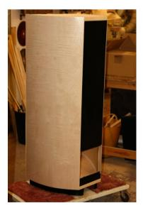
Rear panel fitted. Note the cut-out at the base. This is where I wanted to fit removable crossover panels. I didn't want external crossovers in boxes because of the unwanted extra boxes and wiring.
