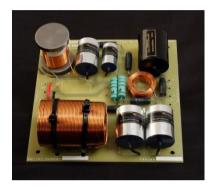
Capacitors are (all bar one) Clarity Cap ESAs. Inductors are from Janzten, the LF and notch filter inductors are air-cored although that's probably overkill. I was careful to ensure electrical compatibility with the originals, so the DC resistance measures EXACTLY as per the Tannoy originals. I had to add a resistor to the notch filter inductor (in series) to achieve the 2.60hms required. PCBs are custom built and fit the space for my removable panels at the rear of the speakers.
