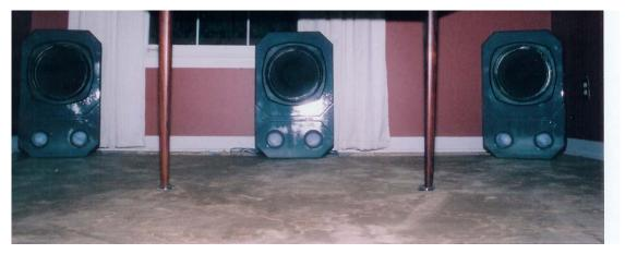
In figure 14 below, we see the 6.0 home theatre located in my basement. I built the wall system which incorporates the speaker. The three drivers you see are all 15 inch diameter Tannoy. The left and right are Monitor Gold which I purchased new in 1972. The center speaker is a HPD385 bought second hand in 2003. With three front speakers of this size, I decided not to use a sub-woofer. The three rear surround speakers (not shown) are all Tannoy Saturn (two 6 inch and one 8 inch).
